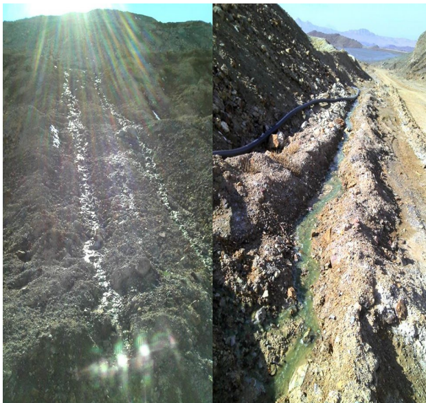
Fig. 8 Seepage of PLS from the eastern slope of the heap, resulting in geotechnical hazards and loss of dissolved copper
